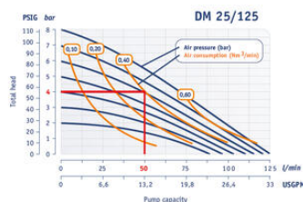
1" Pump - Performance Curve Performance based on water at 20°C
